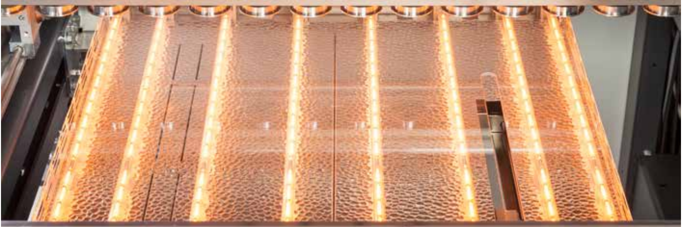
Infrared emitter in the preheating module
