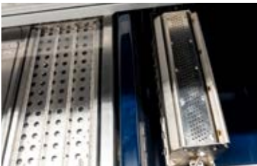
Soldering module: Proven Erska pot technology with a filling volume of only 345 kg
