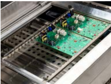
Designed for solder frame operation as standard. Finger transport optional.
