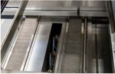
Precise spray fluxer for reliable flux application
