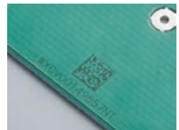
ECU Printed Circuit Board Material: Epoxy Glass
