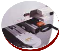
手动调宽数字显示 Manual width adjustment with digital display
