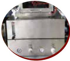
喷雾单元一体化 (可选配选择性喷雾装置) Integrated spray fluxer unit (selective spray device is optional)
