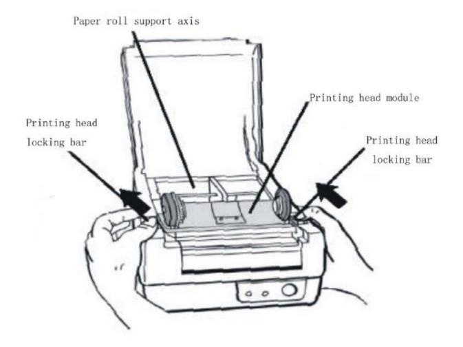
3.4.2 Loosen the printing head's locking bar, open the printing head's module, and adjust it to the vertical location.
