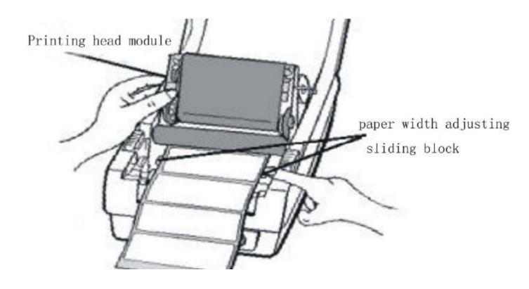
3.2.6 Recover the printing head module, and be sure that the module has been
