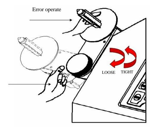
**4.5**. Install the part reel to be counted onto **reeling shaft** on the left, so that the blades on **reeling shaft** are locked to the reel; install temporary reels of corresponding widths on the right; guide the starting part of the tape through the space between **upper guide pole** and **lower guide pole**, press the **guide pulley**, and hang the tractive hole, namely, D in Fig. 1, of the reel onto **counting gear**.
