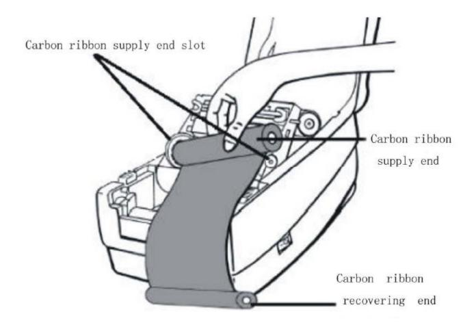
3.4.4 Lock the carbon ribbon recovery end's paper tube into the carbon ribbon recovery end's slot (the step is the same as above), and then slightly roll the gear for a cycle.
