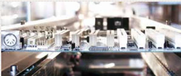
The systems are equipped with electrically width-adjusted conveying systems and center support.
