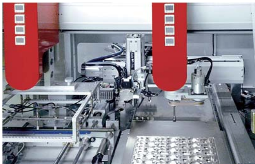
Customized IN-LINE PCB Separator with twin carriers & nozzle module.
