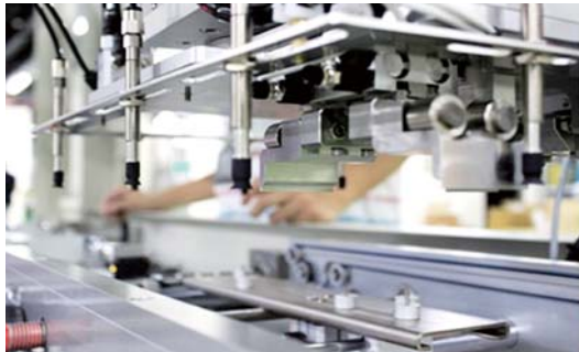
Customized IN-LINE PCB Separator With Customized Grippers & Nozzle pad.
