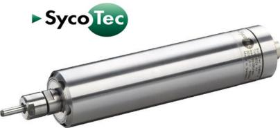
Motor system: 3 phase asynchronous motor Speed range: 5,000~60,000 rpm Voltage: 30V Current: max. 8A Torque: 4.5 Ncm Frequency: 83~1,000 Hz Power: 265W Weight: 700g Bearing system: 2x Hybrid, 1 x Steel, lifetime lubricant Protection category: IP 20 Working position: < Load direction: axial  $\Psi$  radial Run-out (taper):  $\leq 1.5 \ \mu m$ Cooling system: Self-ventilation fan Cooling via clamping bracket Housing material: Stainless steel
