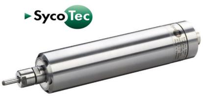
Motor system: 3 phase asynchronous motor Speed range: 5,000~60,000 rpm Voltage: 30V Current: max. 8A Torque: 4.5 Ncm Frequency: 83~1,000 Hz Power: 265W Weight: 700g Bearing system: 2x Hybrid, 1 x Steel, lifetime lubricant Protection category: IP 20 Working position: < Load direction: axial  $\Psi$  radial Run-out (taper):  $\leq 1.5 \ \mu m$ Cooling system: Self-ventilation fan Cooling via clamping bracket Housing material: Stainless steel
