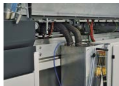
Maintenance "On-the-Fly" continues to operate while the condensation management system is being cleaned
