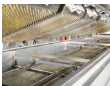
Process tunnel, tested for tightness, guarantees long-term stability
