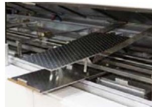
Retractable nozzle sheets for quick maintenance
