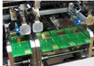
Multi track conveyor for variable PCB width
