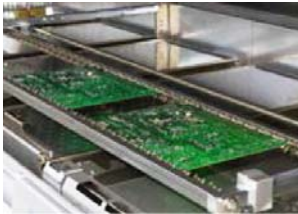
Grip conveyor for extremely thin PCB or flexfoils
