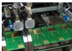
Multi track conveyor for variable PCB width
