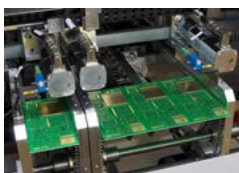
Multi track conveyor for variable PCB width
