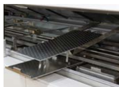
Retractable nozzle sheets for quick maintenance
