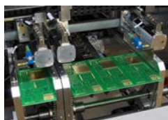
Multi track conveyor for variable PCB width
