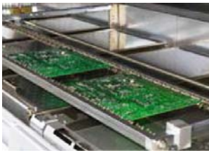
Grip conveyor for extremely thin PCB or flexfoils
