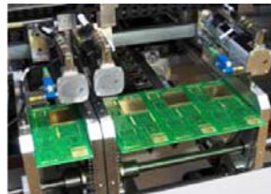
Multi track conveyor for variable PCB width
