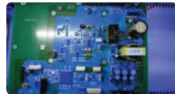
Selective coating on the bottom or top side of PCBA
