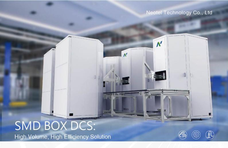
DCS: Distributed Control System. The system adopts distributed control to realize the automation and information interaction of multiple SMD BOXs. Our unique design allows each SMD BOX has its own dedicated controller and work autonomously whilst NeoS still governs all information and monitor material flow all the time.
