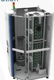
All these steps are automated with SMD BOX SP. It employs a camera to read the barcode information as the first step, then extracting the necessary information like manufacturing date, part number and others then the software will allocate them into Cooling Area with the help of automation mechanics.
