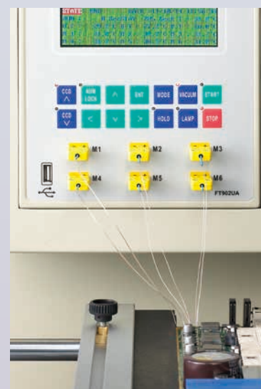
Six Temperature Detectors
