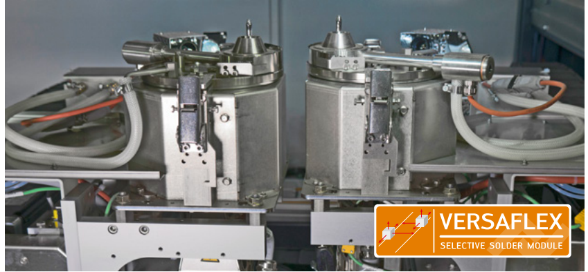
VERSAFLEX module – 2 solder pots mounted on 2 independent axis systems
