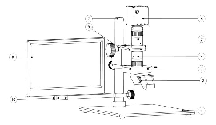
1.stand base 2.2D/3D rotation view 3.4 zones control LED ring light. 4.Zoom body 5.CCD fine focus tube 6.HDMI camera 7.stand post8.Focusing holder 9.19 inch display 10.Arm of display
