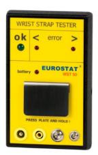
The tester needs to be calibrated yearly. Possibility to calibrate it in-house with calibration plugs ( $10M\Omega$  -  $35M\Omega$ ). Other limits available on request
