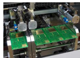
Multi-track conveyor for variable PCB widths
