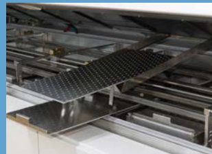
Retractable nozzle sheets for quick maintenance
