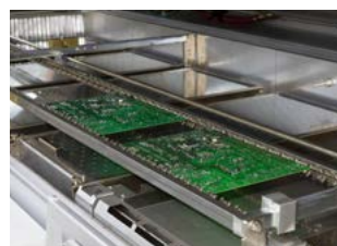
Grip conveyor for extremely thin PCBs or flexible printed boards
