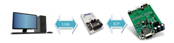
Step 1: Test and save the project (\*dprj) under Dediware engineering mode. Make sure you select "Start from handler" for **start mode** in the **Config** window.
