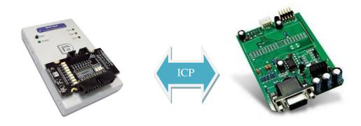
Step 1: Test and save the project (\*dprj) under Dediware **engineering mode**. Make sure to select "Start from handler" for **start mode** in the **Config** window. And use DownPrj to load the project file to the embedded memory.
