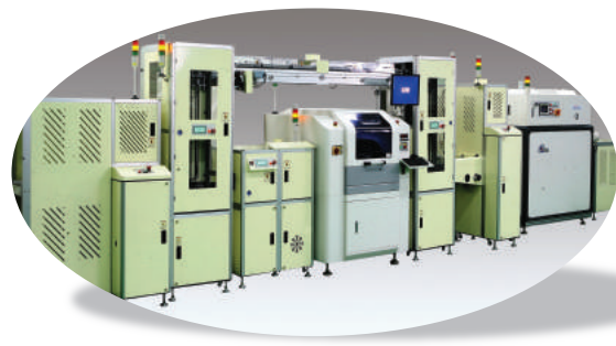
SL Corp. / Automotive •PCB Load – Invert – Coating WorkCell – PCB Unload – Curing Oven – TR Conv. (KL-900Y) (KIV-420Y) (TCM45A) (KU90-900Y) (ECO99C) (TRC-200)
