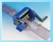
The model SEF 1 is designed for separating wires of flat cables. Two different pitches of separation can be supplied: 1,27 mm (the wires are individually separated Code 73.0L01) or 2,54 mm (the wires are separated by couples Code 73.0L02). This version is a "bench" manual machine suitable for separating edges of flat cables having maximum width of 33mm.
